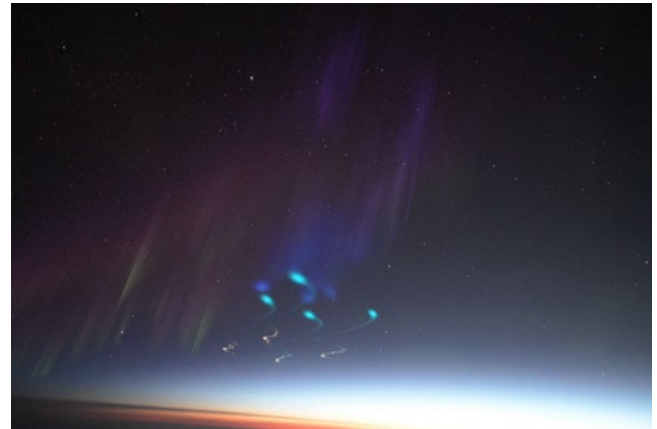
Clouds of vapor traces caused by chemical releases from the C-REX 2 payload form a grid pattern to show the movement of the wind in the upper atmosphere. The photograph was made from a NASA aircraft off the northeast coast of Greenland. Photo by Jason Ahrens.
